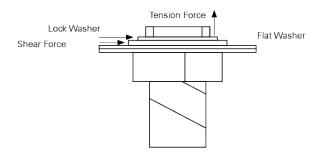
When mounting the FS12TEN loudspeaker to a solid surface use the proper bolts, washers, and lock washers (stainless steel A193 grade B8 is recommended for high strength outdoor installations). Do not substitute mismatched bolts and washers.
